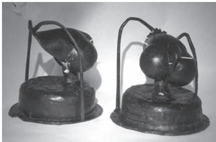
It's always best to weigh the wax at every stage, so you KNOW what each step adds. This is the stage just prior to plaster with sprues, vents, and crucible assemblies.
